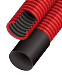
Super Corflo is a dual-wall coilable polyolefin duct, and is the economical choice for conduit and inner duct applications. The dual-wall design offers a light-weight, easy to handle conduit system with an increased crush-resistance, and semi-smooth inner wall for ease of cable pulling. Super Corflo® can be used anywhere Rigid PVC is used: Inner City work (structures), Solar Farms, or any Open Trench work.
